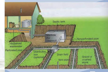
Drainfields treat wastewater by allowing it to trickle from a series of perforated pipes, through a layer of gravel, and down through the soil. The soil is a natural filter and contains organisms that help treat the waste. Solids can damage the drainfield by clogging small holes in pipes and the surrounding gravel. Excess water strains the system unnecessarily.
